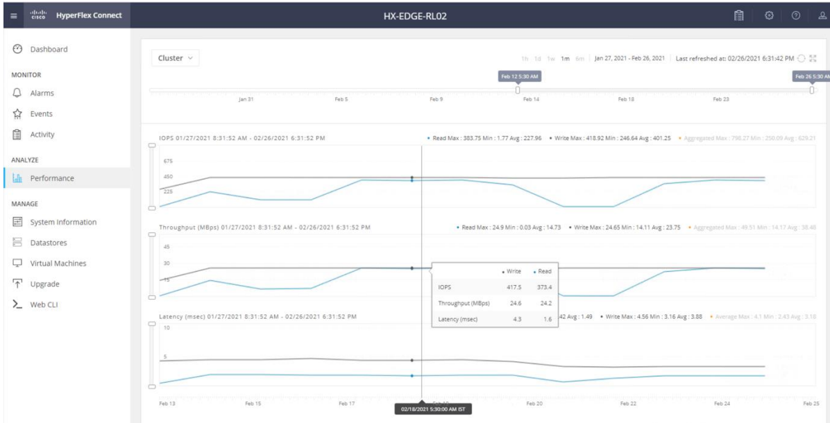
Figure 15. Average read-write throughput and latency of all recording servers observed in Cisco HyperFlex Connect
