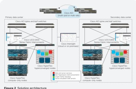
Figure 2 Solution architecture
