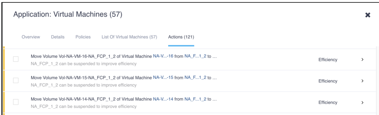
Figure 22. Recommendation to move a virtual machine's volume to a different storage so that a NetApp volume can be suspended
