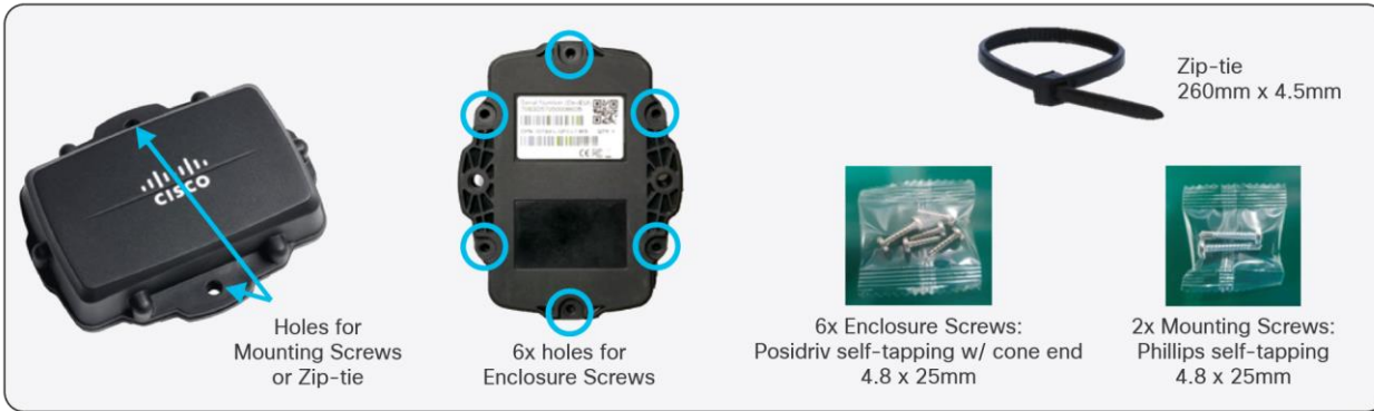
Figure 34. Mounting Accessories and Methods AV300
