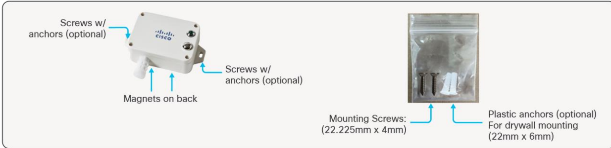
Figure 7. Mounting Accessories and Methods AV201
