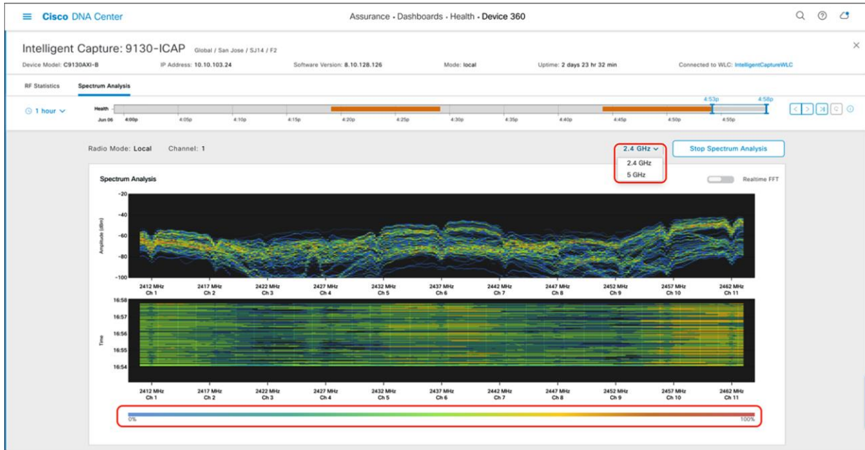
Figure 54. 2.4-GHz Spectrum Analysis with persistent FFT enabled
