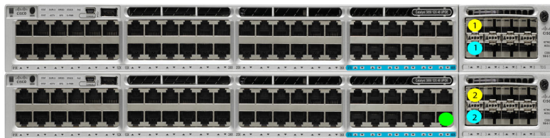
Dual 10/25GE ToR Switches (standalone or stacked)
