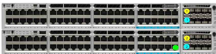
Dual 10/25GE ToR Switches (standalone or stacked)
