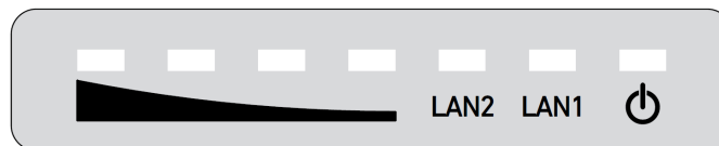
Figure 7. Status and link/boot LEDs
