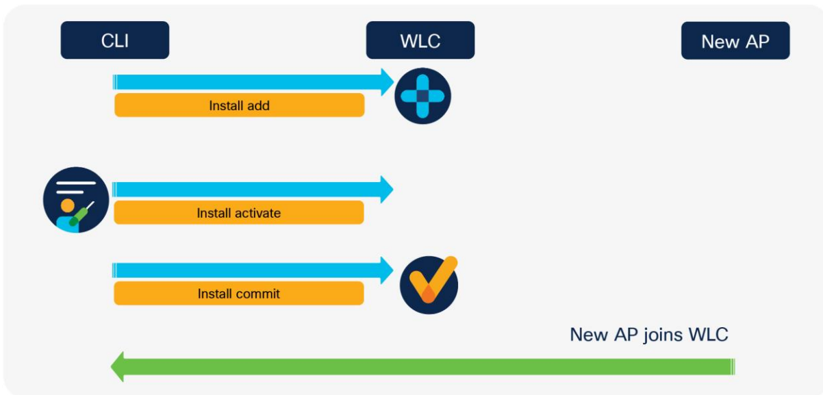
Figure 13. APDP installation workflow
