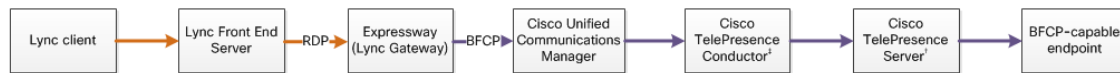
Figure 1: Lync environment to TelePresence Server conference managed by TelePresence Conductor trunked to Unified CM
