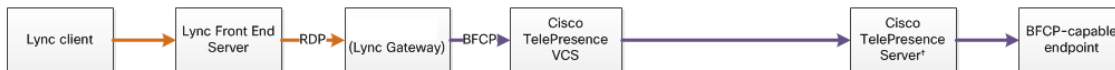
Figure 4: Lync environment to TelePresence Server conference managed by TelePresence Conductor neighbored to VCS
