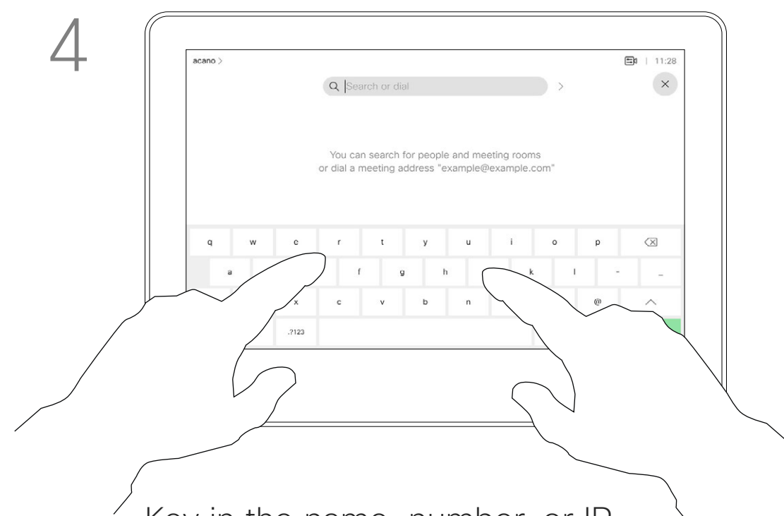
Key in the name, number, or IP address. Matches appear as you type. Tap and hold * to type the point sign used in IP-addresses.
