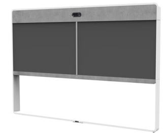
Floor stand secured to the wall
