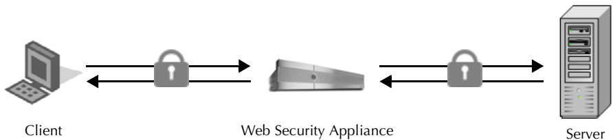
Figure 11-4 HTTPS Connection Decrypted by the Web Security Appliance
