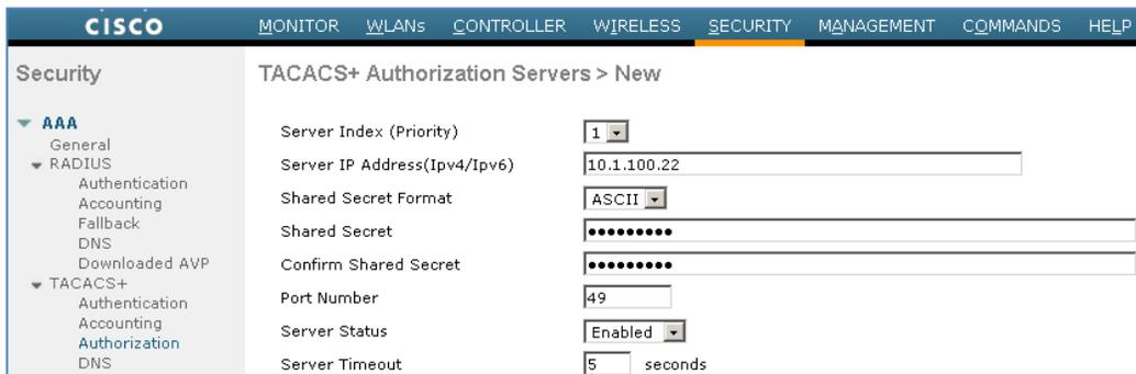
The screenshot shows the Cisco WLC GUI with the 'Security' tab selected. The left sidebar shows the navigation tree with 'TACACS+' expanded to 'Authorization'. The main content area is titled 'TACACS+ Authorization Servers > New'. The configuration fields are as follows:
