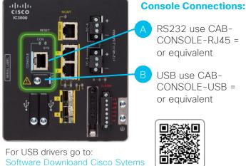
3 Connect a network cable from your PC to the MGMT ENET of the IC3000.
