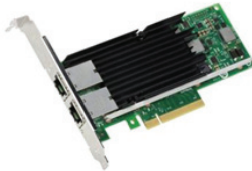
Figure 7. Intel® Ethernet Converged Network Adapter X540-T2.
