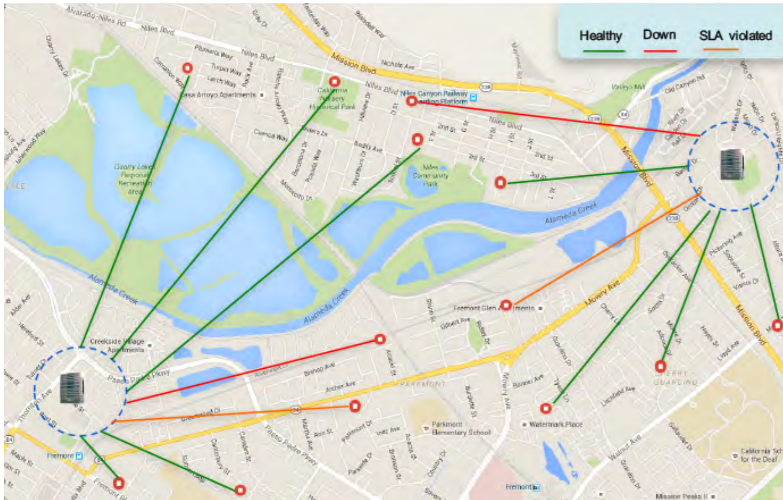
Figure 5. Cable Network Management
