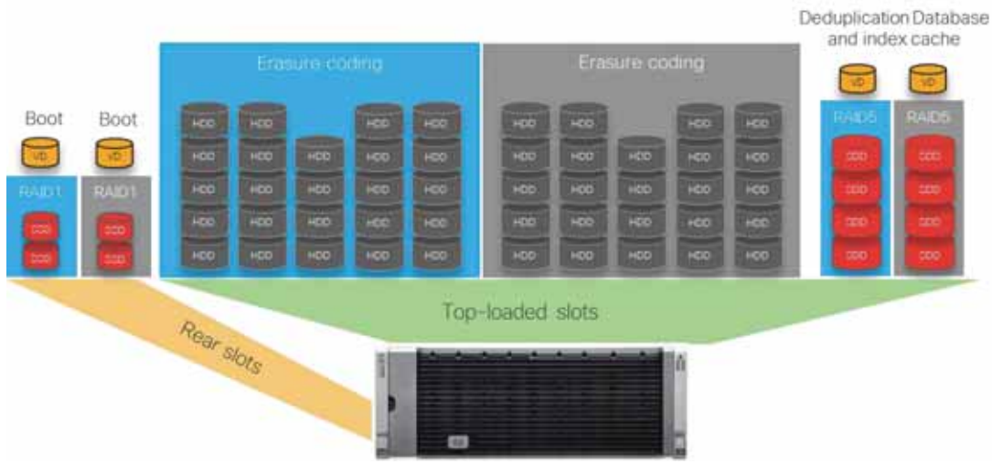
Figure 7. Cisco UCS S3260 storage layout
