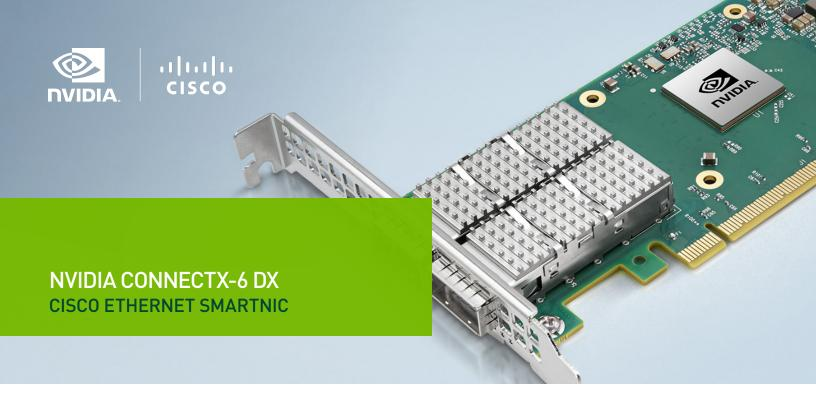
NVIDIA® ConnectX®-6 Dx is a highly secure and advanced smart network interface card (SmartNIC) to accelerate mission-critical data center applications, such as security, virtualization, big data, machine learning, and storage. It provides two ports of 100Gb/s Ethernet connectivity and the highest ROI of any SmartNIC.
