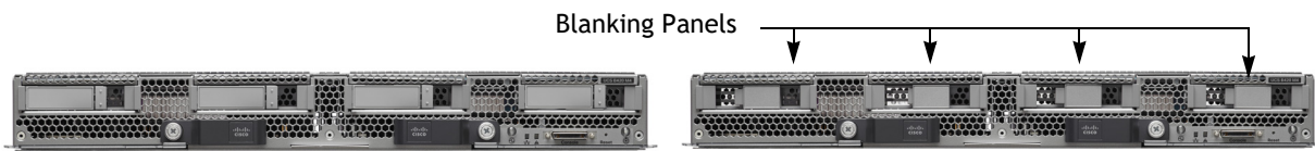
(a) Server with four drive bays
