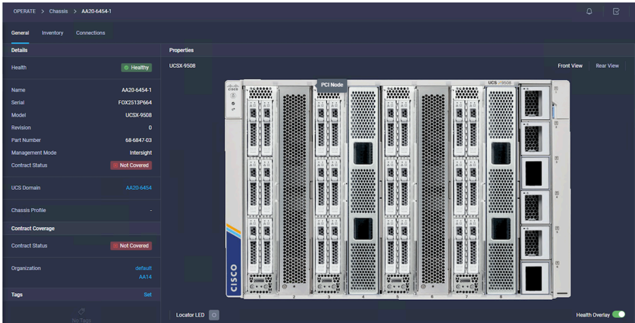
Figure 9. PCIe nodes in slot 2 and slot 6 next to X210c Compute Nodes in slot 1 and slot 5
