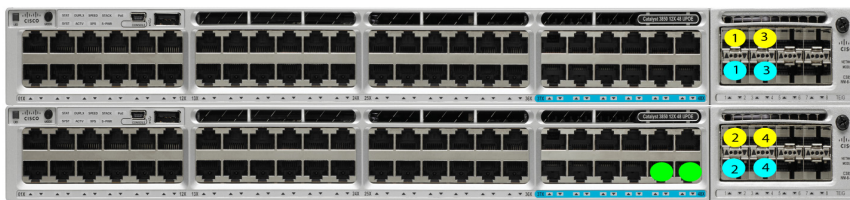
Dual 10/25GE ToR Switches (standalone or stacked)
