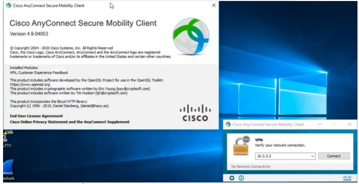
msiexec -i anyconnect-win-4.9.04053-umbrella-predeploy-k9.msi TRANSFORMS=\_anyconnect-win-hide-addremove-display.mst ARPSYSTEMCOMPONENT=1 -lvx\* install.log
